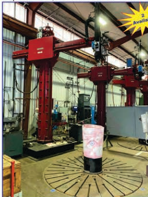
Clad Unit #1: A&N Plant Model RC40X3.75 Cladding Machine with Arc Specialties Hot One Solid State Hotwire Power Supply and Esab 350 MPI MIG Welder
