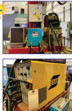
Clad Unit #1: A&N Plant Model RC40X3.75 Cladding Machine with Arc Specialties Hot One Solid State Hotwire Power Supply and Esab 350 MPI MIG Welder
